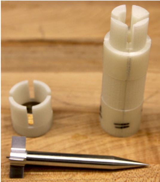
Fig. 5 Prototype projectile and sabot components.
